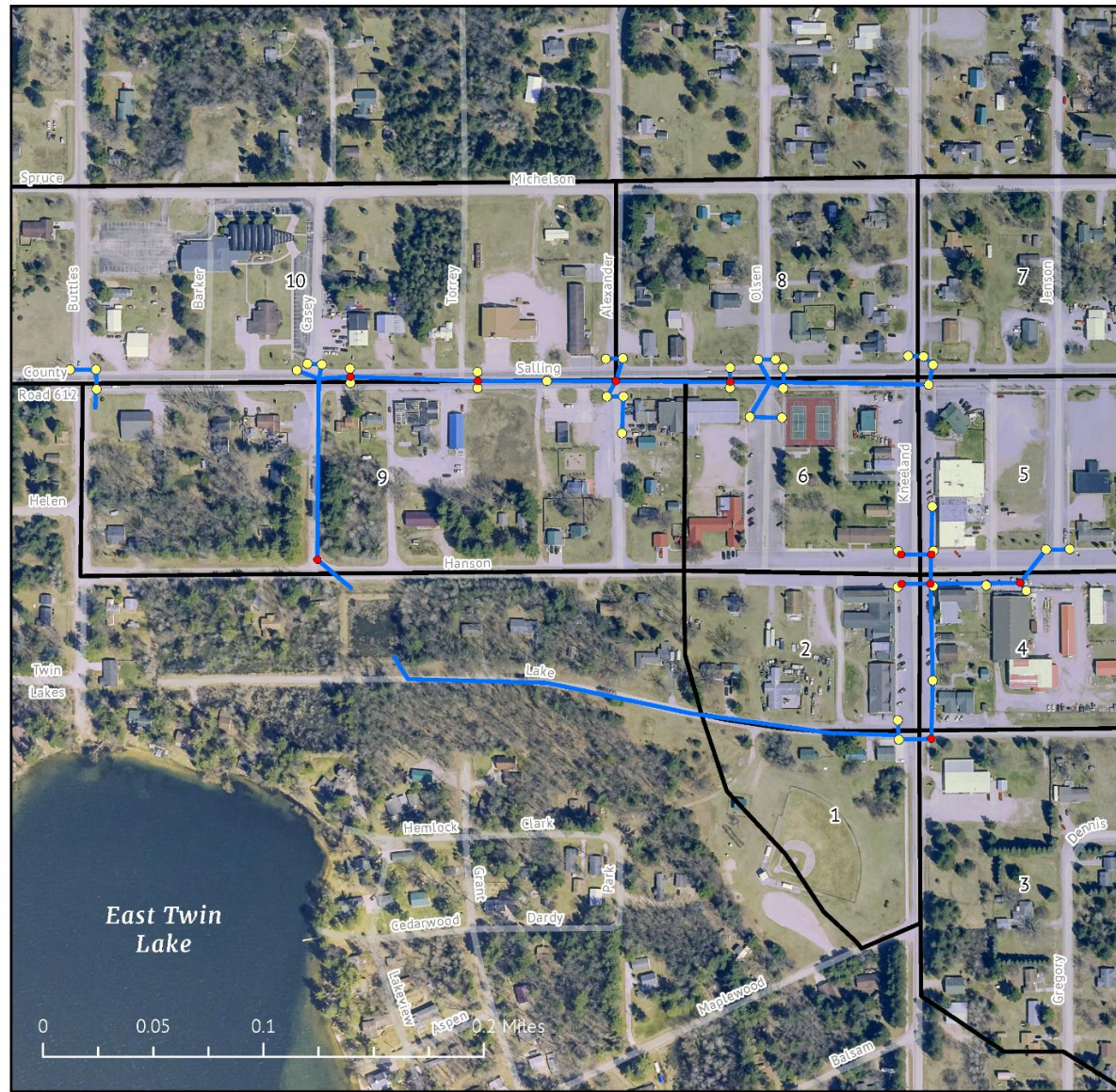
Figure 3. Current underground stormsewer system in Lewiston, MI.
